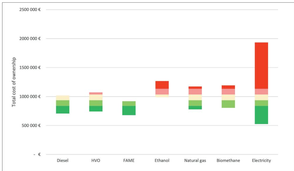
**Figure 21.** The total cost of ownership during the 10 years of use. The colors indicate how the costs relate to the scale of the indicator (dark green = Very Good, dark red = Very Poor). Based on Dahlgren and Ammenberg (2021).
