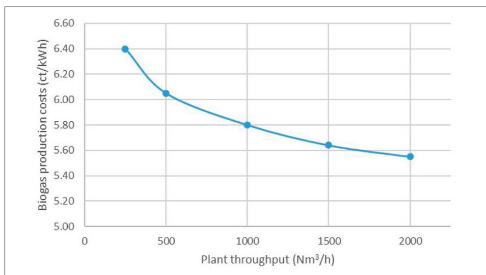
**Figure 18. Biogas production costs (euro cents) with increasing plant size for a biogas facility co-digesting maize and slurry (90% maize, 10% slurry). Data from IRENA (2018).**
