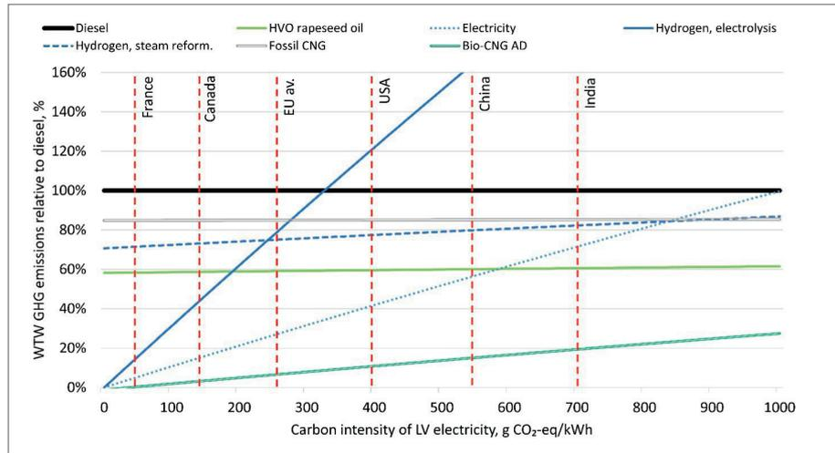
**Figure 23. Well-to-wheel greenhouse gas emissions (relative to diesel) of energy carriers for a suburban bus, as a function of carbon intensity of the electricity system. Based on Gustafsson et al. (2021).**
