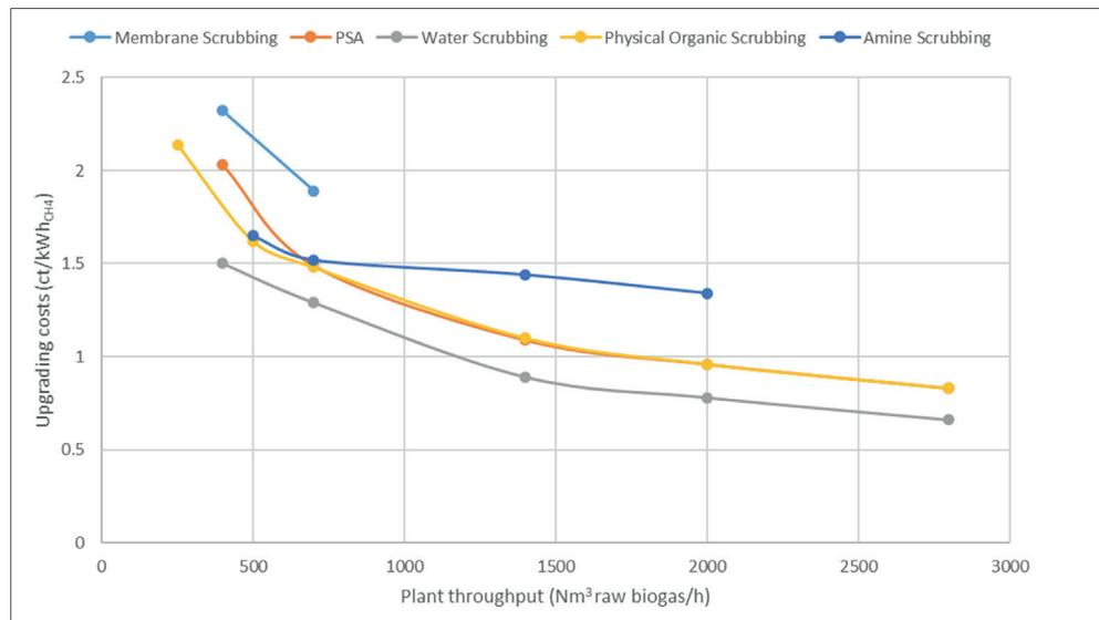
**Figure 19. Specific costs (euro cents) for biogas upgrading technologies. Data from Billig et al. (2014).**
