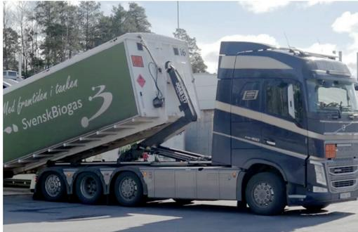
**Figure 10.** Example of a swap body transport in Linköping, Sweden. The container holds compressed biomethane at 200 bar. In this case the truck used is fueled by liquid biomethane. It is a Volvo, 460 hp.
