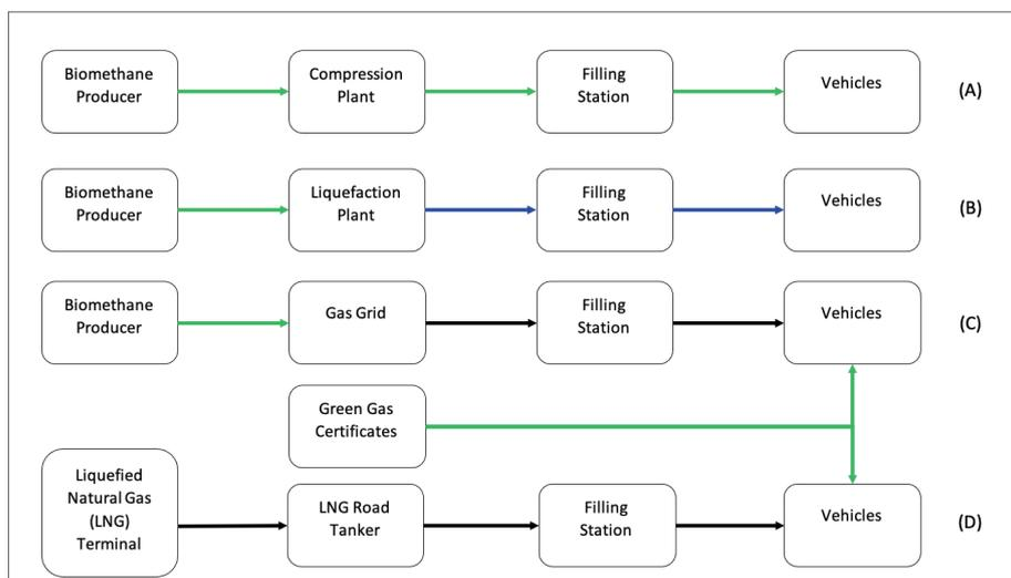
Figure 14. Biomethane supply chains to filling stations. (A) Direct connection to biomethane producer, compressed biomethane. (B) Direct connection to biomethane producer, liquefied biomethane. (C) Compressed biomethane via gas grid and green gas certificates. (D) Liquefied biomethane and green gas certificates.
