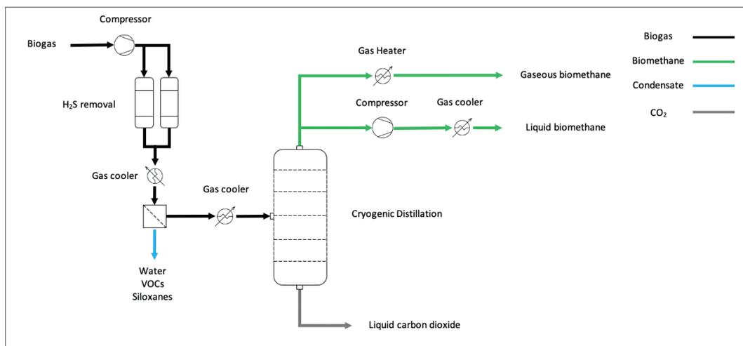
Figure 7. Cryogenic separation system topology.
