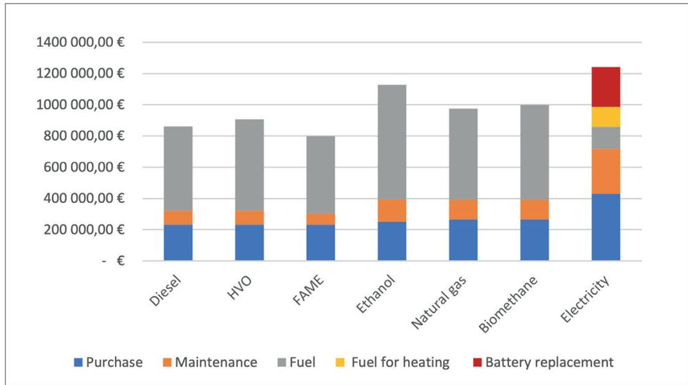
**Figure 20.** The total cost of ownership divided into costs for purchasing, maintenance and fuel/electricity. The numbers are mean values between the lowest and highest found costs for each part. Based on Dahlgren and Ammenberg (2021).
