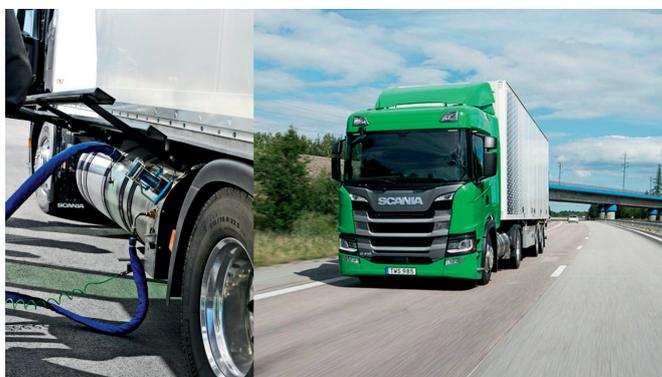
**Figure 32. A biomethane powered truck from Scania to the right. To the left, a truck is filled with liquid biomethane.** Photos taken by Peggy Bergman, Scania CV AB and Mirja-Lisa Niemi, Klara Språket.
