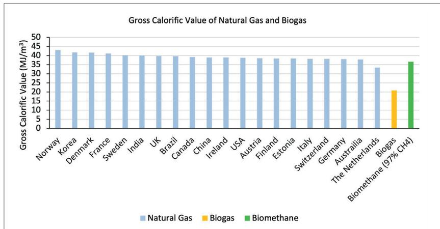
**Figure 2. Gross calorific value of natural gas and biogas (55%<sub>vol</sub> CH<sub>4</sub>).**
