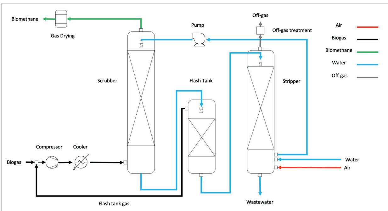
Figure 3. Water scrubbing system topology.
