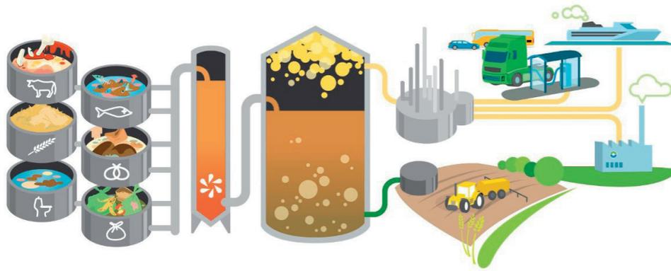
**Figure 1.** A schematic illustration of biogas solutions, where different types of feedstocks are converted in AD plants to biomethane fuel and biofertilizers for use in agriculture. In addition, carbon dioxide is separated and may be used for different purposes. *Illustration: Mattias Schläger.*
