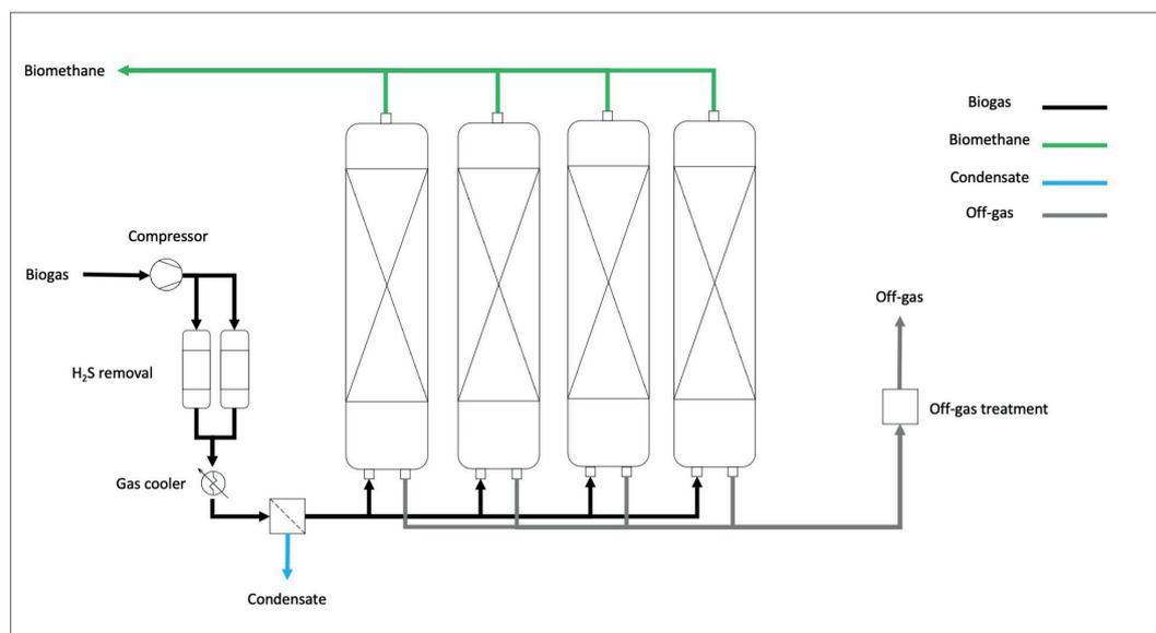
Figure 5. Pressure swing adsorption system topology.
