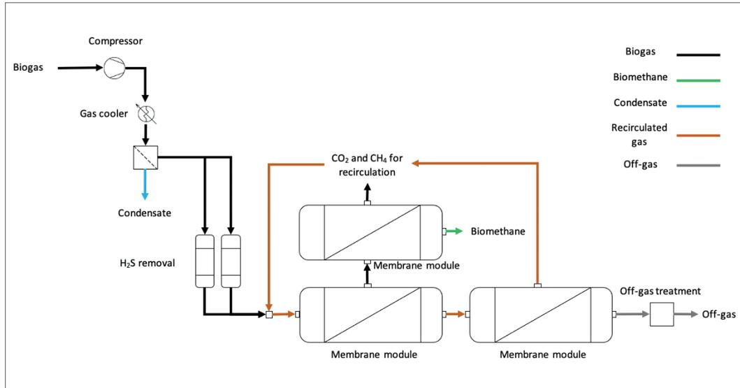
Figure 6. Membrane separation system topology.
