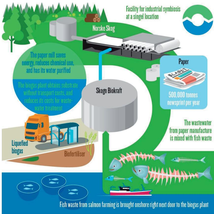
**Figure 26. Illustration of the industrial symbiosis system at Skogn, where the biogas plant is an important cornerstone.**
