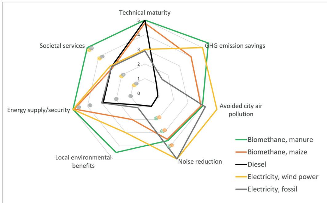
**Figure 37. Schematic illustration of multi-criteria analysis results for two types of biomethane, in comparison with two types of electricity and fossil diesel. Alternative results presented with pattern filled circles, which indicates larger uncertainties.**
