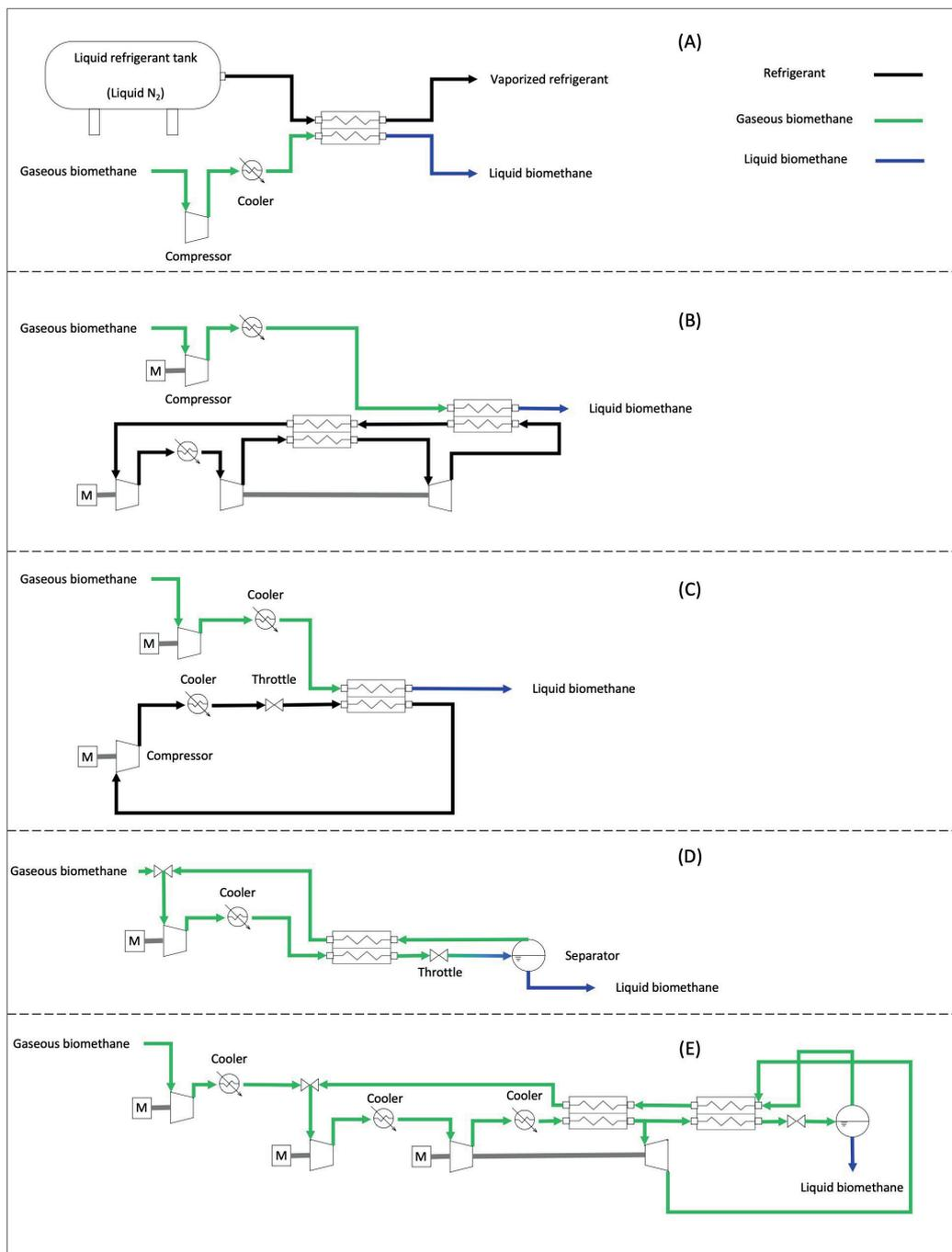
Figure 8. Biomethane liquefaction: (A) Liquid nitrogen vaporization, (B) Reverse Brayton cycle, (C) Reverse Rankine cycle, (D) Linde Cycle, and (E) Claude cycle.
